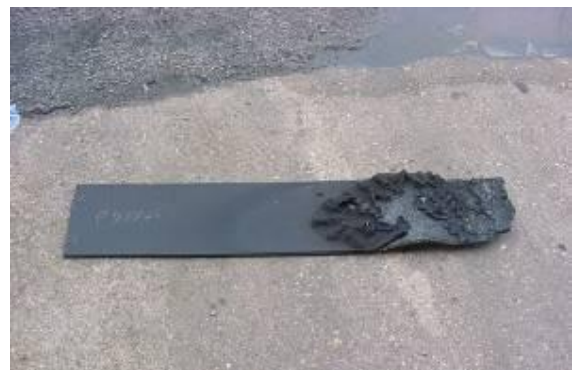
Belt sample after drum friction test
